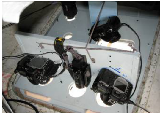
Figure 3. BOSS 2012 Russian survey aircraft (Antonov AH-38-100) and camera setup showing a downward facing Nikon D3X and two oblique Nikon D300s. The cooled thermal imager, Malahit-M, is in a separate compartment of the aircraft.
