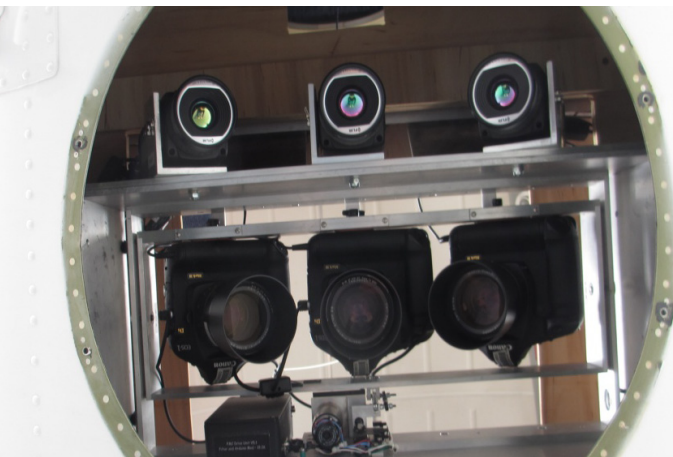
Figure 4. NOAA Twin Otter (right) with belly port camera setup: three Canon 1Ds Mark III dSLR cameras paired with three FLIR SC645 thermal imagers.
