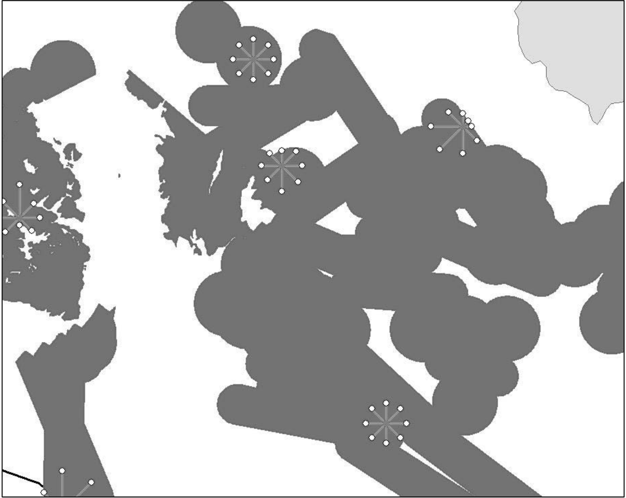
Figure 5. Example of 1-km transect plan lines for remote operated vehicle (ROV) dives. Plan lines have been adjusted in some cases to remain within the delineation of rocky habitat (solid gray).
