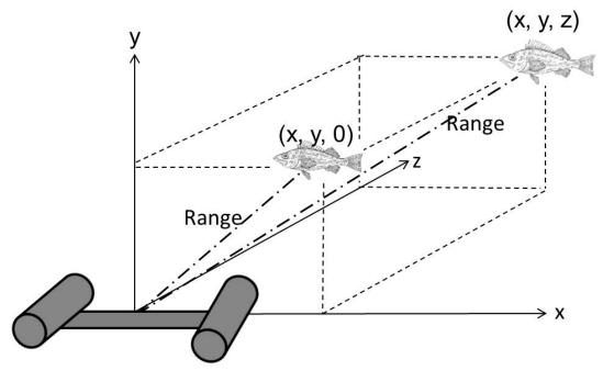
Figure 7. The components of a 3D point measurement.
