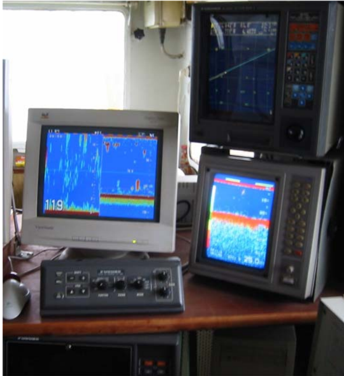
Figure 2. The on-board fish-finding acoustic equipment.
