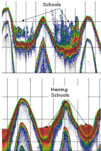
Figure 6. Example echograms of herring distributions observed at 38 kHz during November (A) and February (B) in Lynn Canal, Alaska. Depth intervals are displayed at 50-m increments, and horizontal cells are separated by 0.1 nmi. Herring schools are clearly more dispersed and shallower in November, whereas herring form dense schools in the deep trenches during February. The green thin line represents the seafloor.
