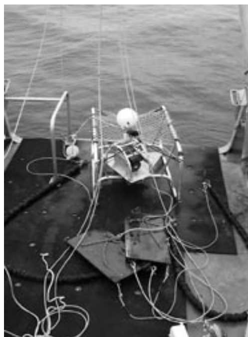
Figure 1. DIDSON sled ready for deployment. Pictured are the aluminum benthic sled with the forward mounted DIDSON (black box), sweeps and doors. The sled is equipped with a light meter as well as a 'pinger' to aid in recovery should the sled become hung on the bottom.
