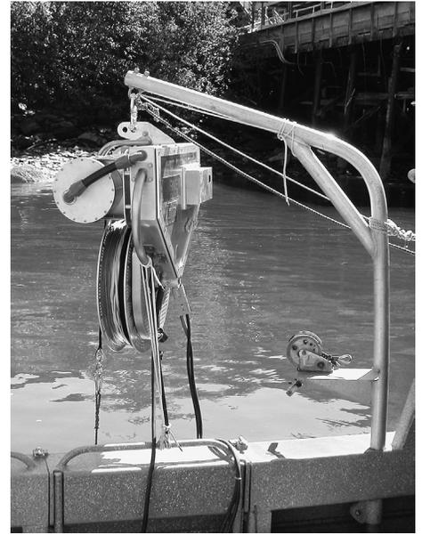
Figure 2. The Sidewinder block winch suspended from a davit on a 24' research vessel.
