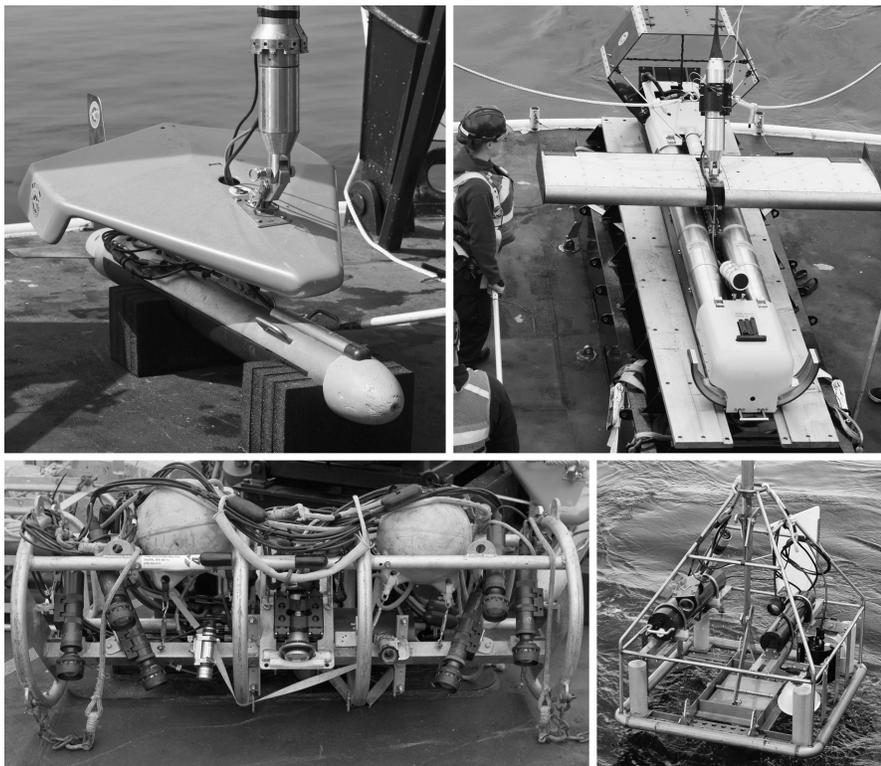
Figure 10. Towed scientific and hydrographic instruments that require subsea positioning capability (clockwise from upper left): Klein 5410 side scan sonar, Klein 7180 long-range side scan sonar, SEABOSS sediment grab/camera system, and the two-part TACOS video sled. SEABOSS was not included in this exercise because of acceptable performance during the 2009 FISHPAC-project cruise in the EBS.
