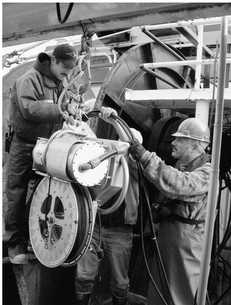
Figure 1. The Sidewinder block winch, showing aluminum housing of the drum below the (left to right) planetary reducer, brake, line guide, motor, and lifting handles above.
