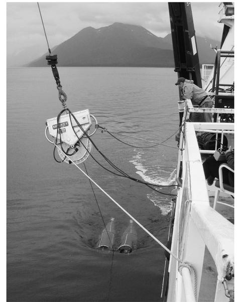
Figure 3. A Bongo net being retrieved by the Sidewinder block winch suspended from a midship boom on a 165' vessel. The remote control operator is partially visible at right, and the net is retrieved through a “barn door” by the scientist below in the hardhat.
