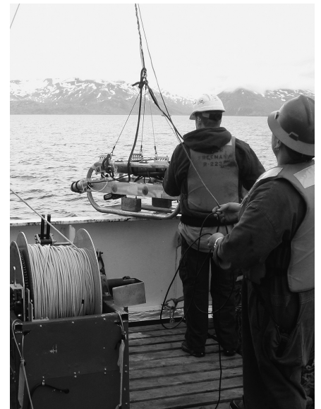
Figure 4. A towed video camera system aboard the NOAA ship Miller Freeman is deployed during a study of untrawlable grounds in the eastern Aleutian Islands. Photo by Frank Shaw.
