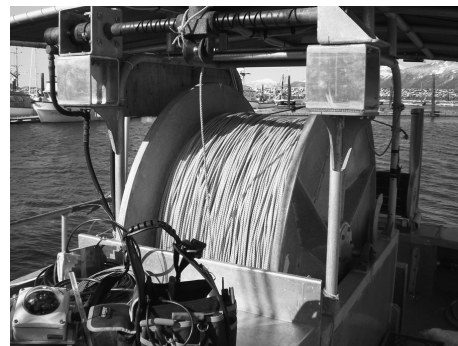
Figure 1. Electronic monitoring gear (foreground) being prepared for installation on a longline vessel. One of the video cameras that will be mounted to the vessel is in the lower left corner.
