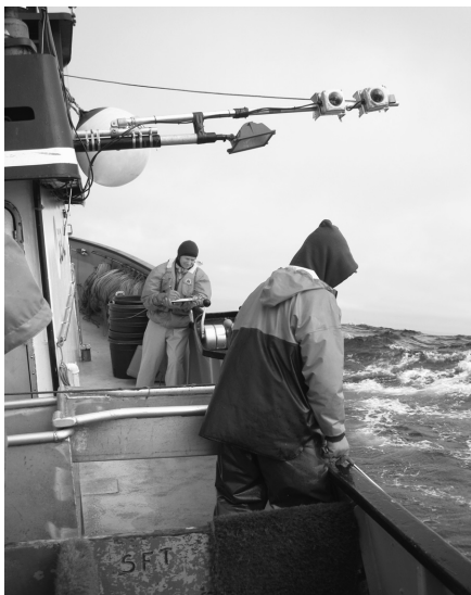
Figure 2. An observer (facing camera) collects data while two cameras, shown in the upper right quadrant of the image, videotape fish captured on longline gear.
