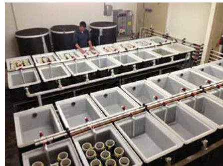
Figure 3. The current iteration of the Cold Water Research Lab incorporates 32 tanks for studying the effects of water temperature on fish and crab growth. Water can be chilled down to 0°C, to study Arctic species. The lab was designed with flexibility in mind, to allow for various sized tanks and precise control of ambient illumination and photo periods.
