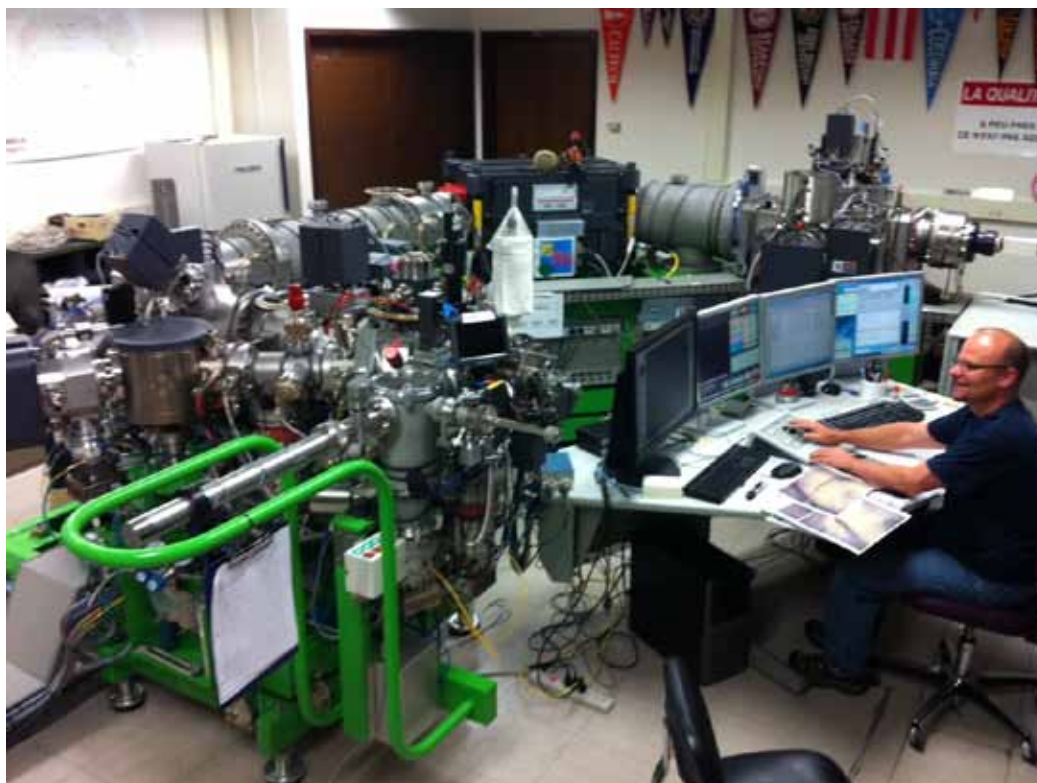
Figure 1. The University of Wisconsin-Madison Secondary Ion Mass Spectrometer (WiscSIMS) IMS-1280 ion microprobe. Dr. Thomas Helser, Age and Growth Program Manager, is at the helm.
