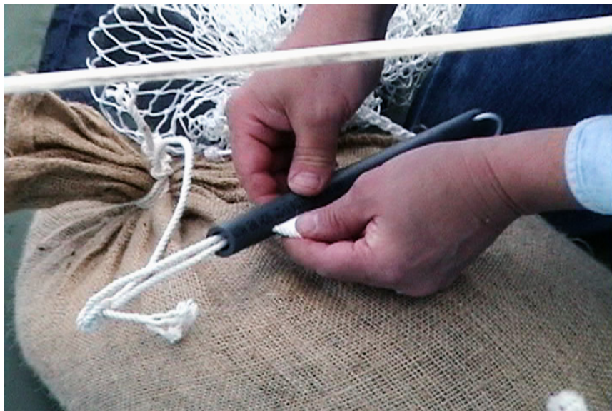
Figure 5.-- Corroding link weight release device.
