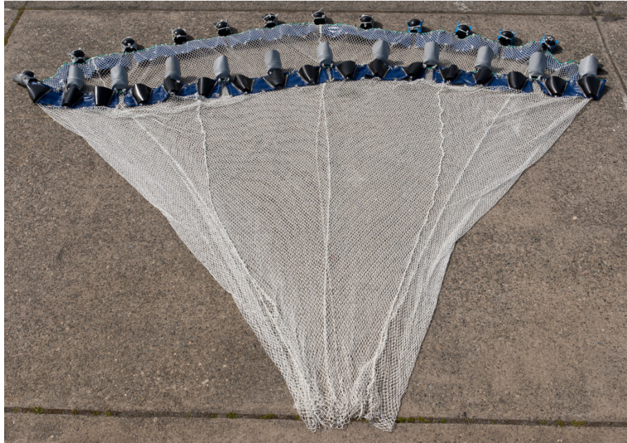
Figure 6. -- Free vehicle trawl with 8.4 m 2 mouth area.
