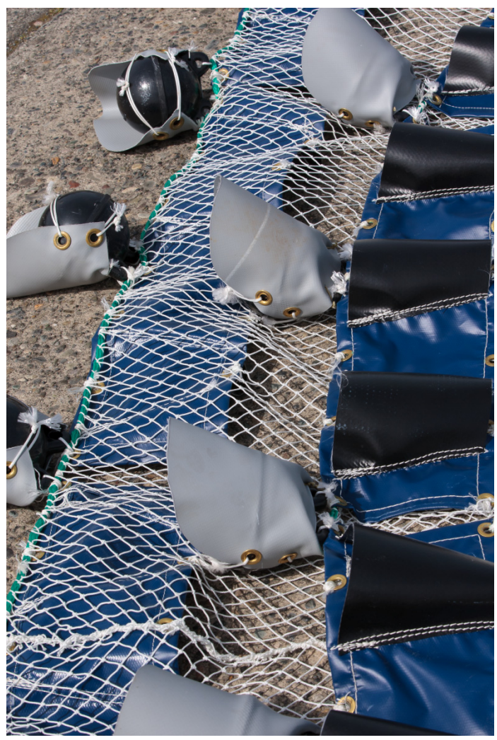
Figure 4. -- Finned trawl floats and hydrofoil kites on mouth rope.
