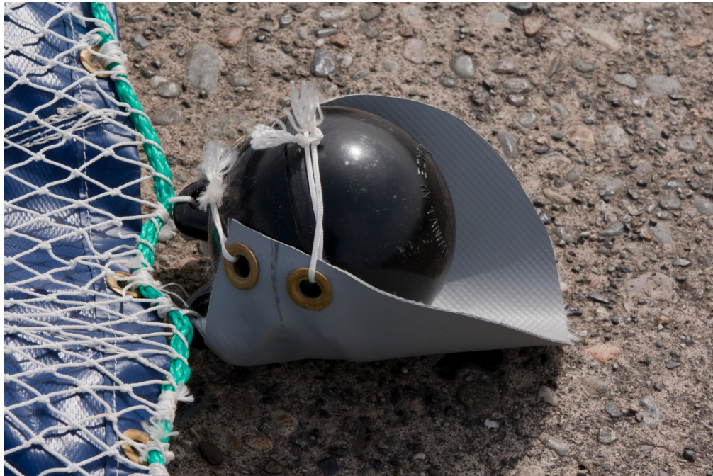
Figure 2. -- Finned ½ liter trawl float.
