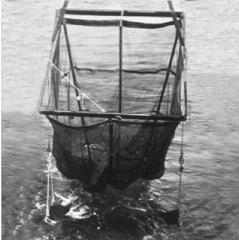
Figure 1. Methot frame trawl with the Isaacs-Kidd depressor (Methot 1986). Methot, R. D. 1986. Frame trawl for sampling pelagic juvenile fish. Calif. Coop. Oceanic Fish. Invest. Rep. 27:267-278.
