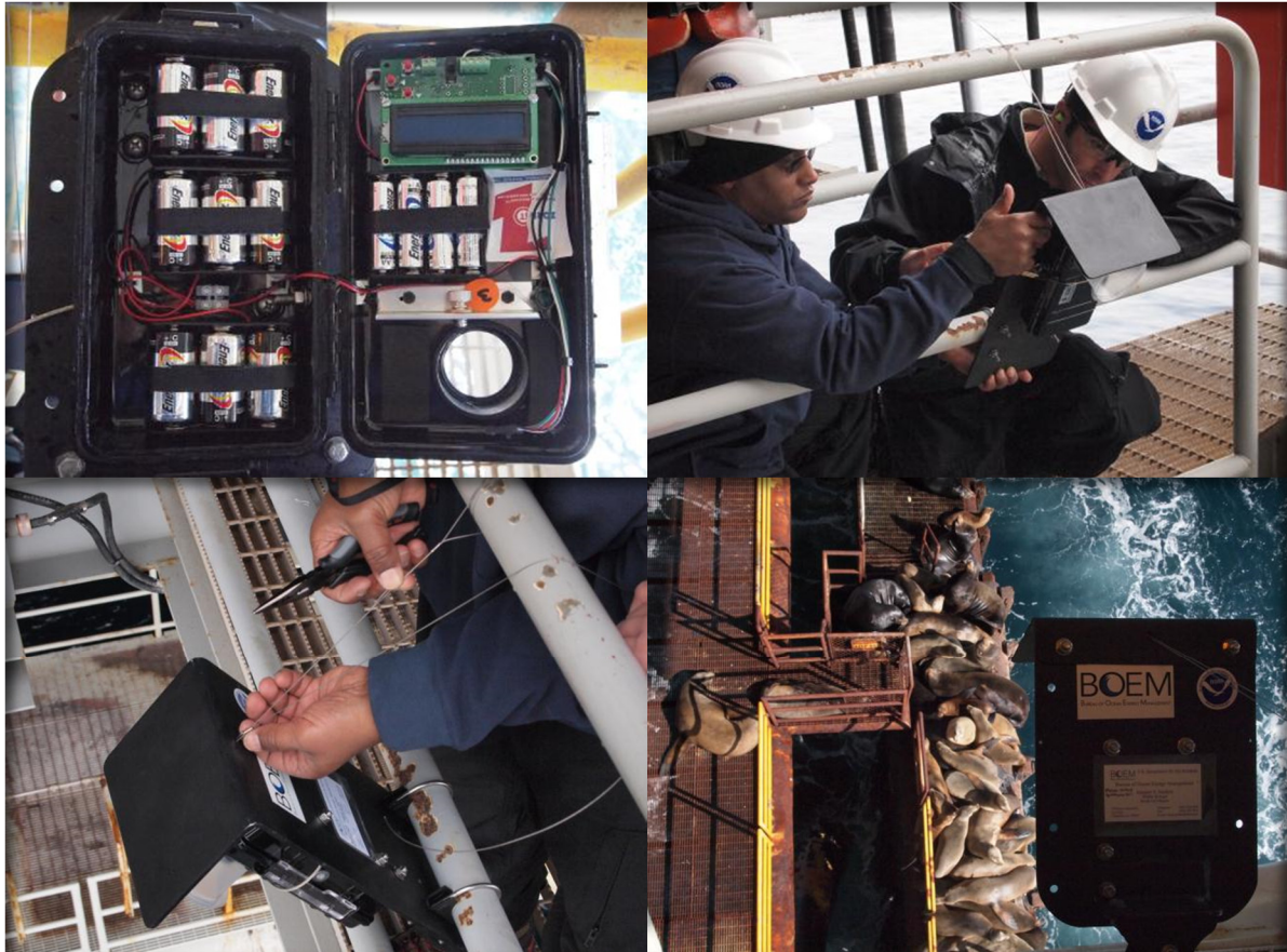
Figure 3. -- Digital automated time-lapse camera systems (developed by Trail Watcher Game Cameras; Monticello, Georgia) that were installed on five gas and oil platforms offshore southern California and programmed to take images between January 2013 and January 2015. The systems consisted of a timing circuit, a camera, and battery bank. They were placed in locations where most areas where pinnipeds could be viewed were covered.
