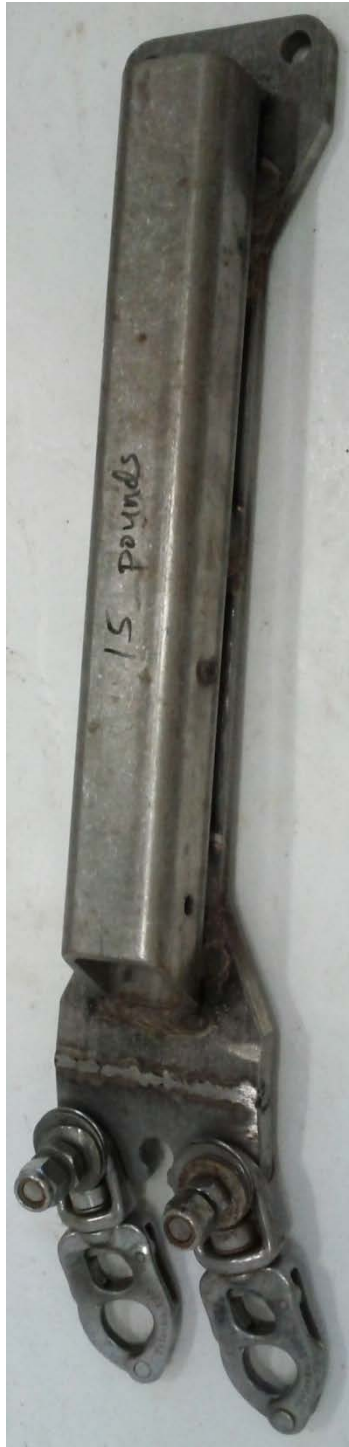
Figure 2f. - - The bottom contact sensor and its footrope attachment configuration to the ground gear used during the 2016 EBSS survey.
