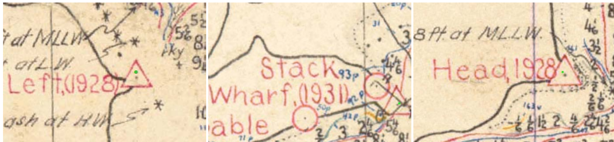
Figure 14. -- After georegistration and datum-shifting, triangulation stations Left (A), Wharf (B) and Head (C), all show close alignment with the independent file of NAD83 HARN triangulation stations.
